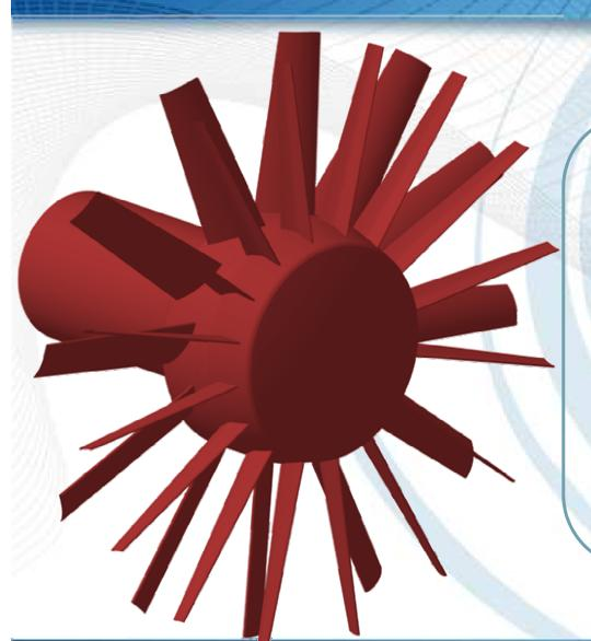
Geometry at hands consist in two row of an axial fan sizing 1744mm at shroud, wile 700mm at hub. The resulting geometry is an assembly of two row, a stator and a rotor fan spinning at 750rpm. The attained speed corresponds to have an axial flow of 612kg/s producing an axial velocity of 53.4m/s. Since no geometry of the stator existed as 3D model, Numitalia provided a starting point geometry defined by means of velocity triangled based on free vortex theory
